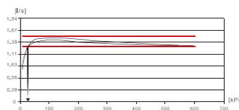
Schematic view of the flow development for cartridge type 40, 952-000-4014176. Nominal flow 1.388 l/s (+/-5% red lines). The cartridge is in the pressure range at 23-600kPa.
